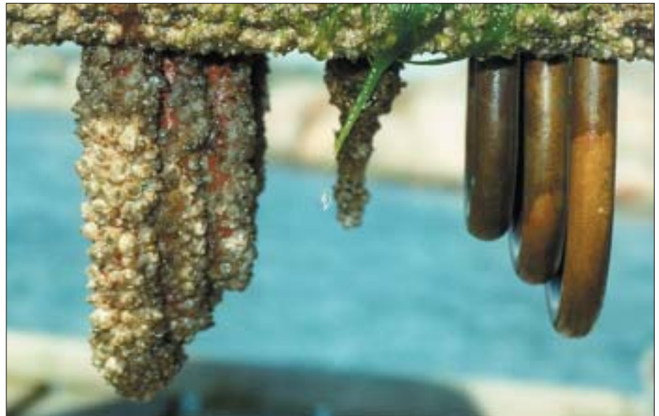
Protection against bio-fouling is necessary, but copper-nickel alloys is naturally protected. The left part of the picture shows a traditional coated boxcooler, the right part with tubes of copper-nickel
